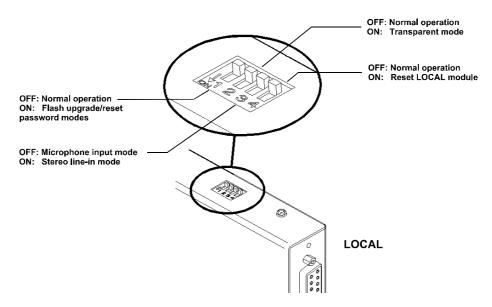
Note: When shipped, all switches are set in the OFF positions and this will produce normal operation with normal microphone input (at the REMOTE module.)
